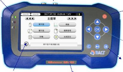
TFT 5 inches color display Resistive touch panel IP 65 waterproof design
